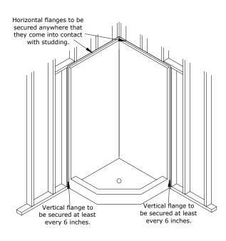
IF A BEDDING MATERIAL IS USED UNDER A UNIT; CEMENT SLURRY, THIN MORTAR MIX, PLASTER OF PARIS, OR A COMPARABLE FLOOR FILLING COMPOUND THAT IS NOT WATER SOLUBLE ARE PROPER BEDDING COMPOUNDS. WATER SOLUBLE MATERIALS, FOAM AND OTHER EXPANDING MATERIALS ARE NEVER TO BE USED AS A BEDDING COMPOUND.
